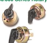
The 700 and 800-Series are single pole multi-position, general purpose rotary switches. These switches feature a nylon actuator in a metal clad construction along with a self-cleaning silver plated contact design. The 700 and 800-Series are typically used in applications requiring multi-position speed controls, such as electric fans.
